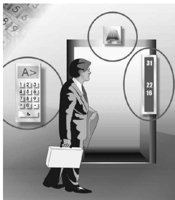
Figure 1: A telephone-like ten-digit keypad allows passengers to enter their destination before they enter the elevator. A display informs passengers of the elevator to which they have been allocated.
