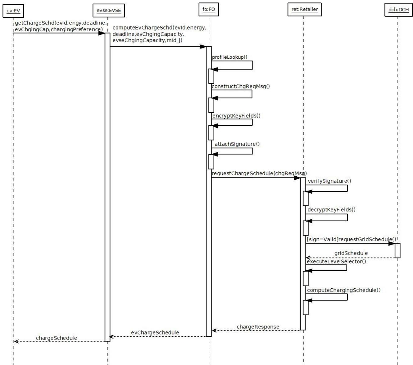
Figure 2: Simplified sequence diagram for EV smart charging request
