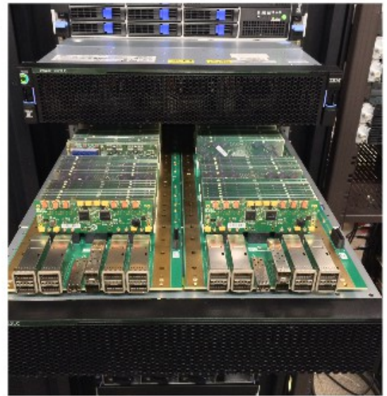
Figure 2: Block diagram of the PCB interconnect (left) and photo of two sleds in a chassis (right).
