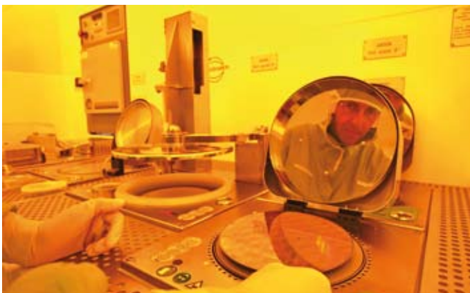
Wafer processing in the lithography section of the cleanroom
